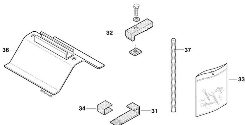
DISPOSITIF DE MONTAGE SUR TOITURE - TÔLE OU BARDAGE - COLIS EG 23
