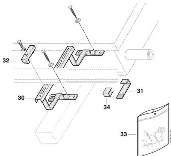
DISPOSITIF DE MONTAGE SUR TOITURE - TUILES PLATES OU ARDOISE - COLIS EG 18, EG 21, EG 44, EG 45, EG 46
